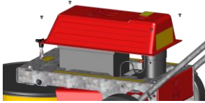
Abb. 12: Demontage Haube WR 870 Akku
