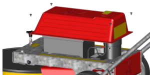
Fig. 12: Disassembly of the WR 870 battery bonnet
